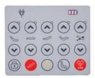
Nurse Side Embedded Controls provide features such as Motorized CPR and Emergency Head low along with the ability to lock certain functions
